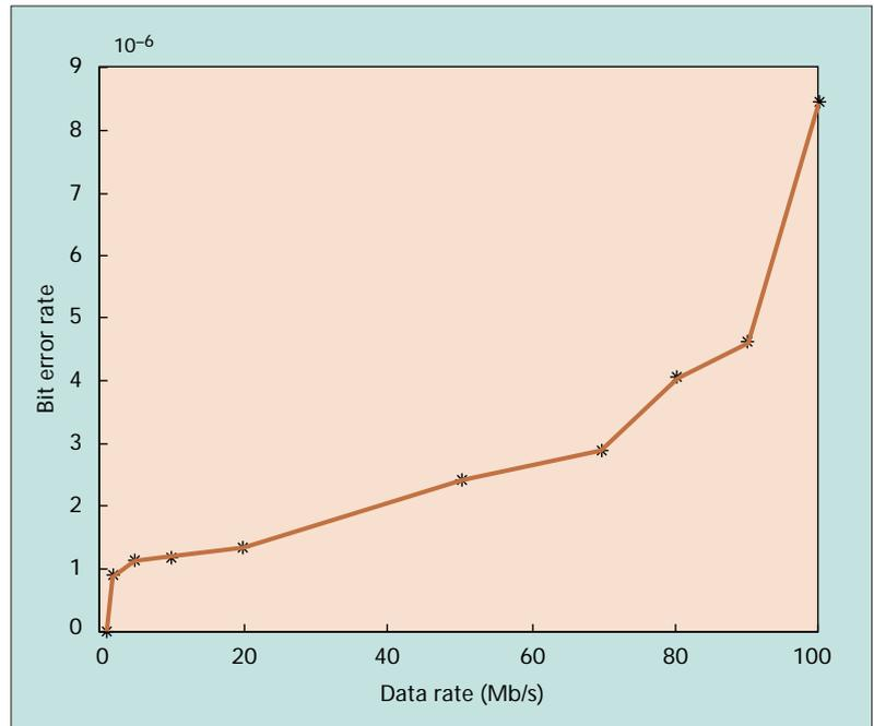
■ Figure 3. BER due to the topology control process.
