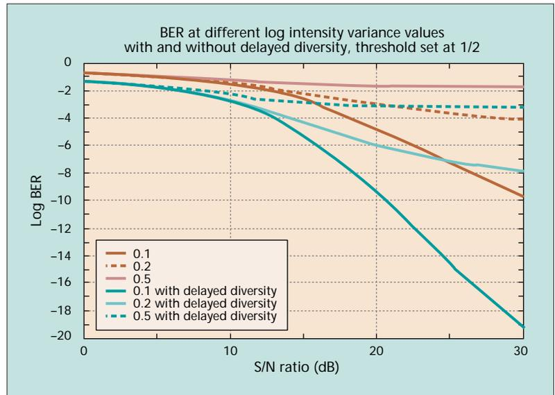
Figure 1. Variation in BER for a 1 km link operating at 1.3  $\mu$ m at 1 Gb/s with and without the use of time-delayed diversity.
